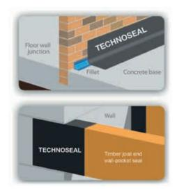
Technoseal is a SBR latex-based liquid applied membrane for waterproofing applications. Available in black and white.
