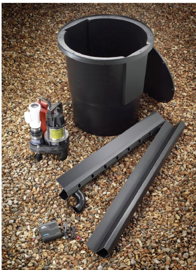
control water ingress. The system consists of a pre-formed polyethylene sump basin, a mains powered 240v submersible pump, a non-return valve assembly and a battery operated high water level alarm, which is linked to an integral float switch. **The WYKAMOL AQUA PUMP** system can be used to de-water the ground or additionally linked to **WYKAMOL AQUA CHANNEL** (see WYKAMOL Aqua Channel Data) relieving water ingress from retaining walls and in turn pumping out to a suitable drainage point.
