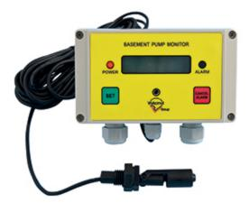
Designed to monitor automatic water sump pumps, it is wired in the power line to the pump. It also has the option to add a high level water alarm indicator. A built-in alarm relay can signal a home automation system, house alarm or a remote dialler.
