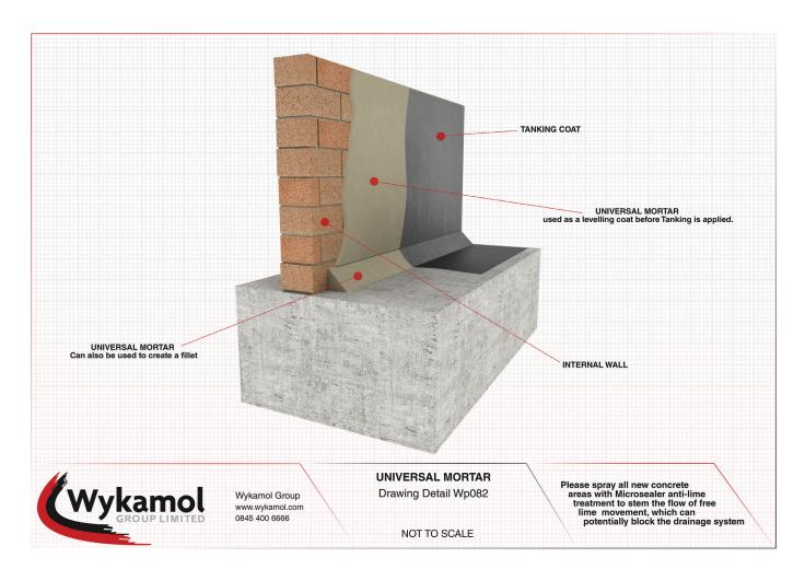
If you are using Wykamol Tanking Slurry on a brick or stone built wall please make sure you use HydraDry Universal Mortar, as a levelling coat for preparation as per diagram.
