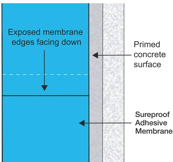
5. At a top angle or corner the horizontal membrane should overlap onto the vertical (See Fig 12).
