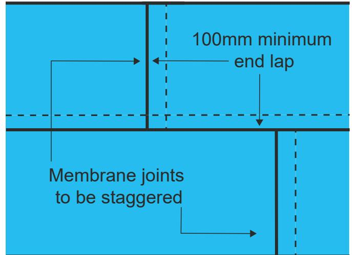
6. End-of-roll overlaps of adjacent lengths should be staggered to avoid them being side by side on adjoining rolls, causing a four fold overlap (See Fig 1).
