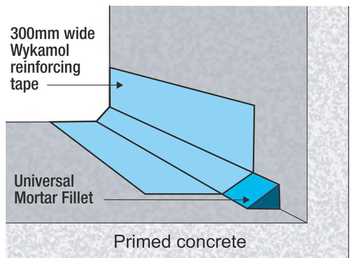
All internal & external angles should be reinforced with Sureproof Reinforcing Tape 300mm wide, centred along the corner angle.
