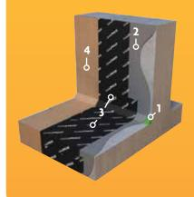
The adhesive surface is protected by a disposable paper interleaving wider than the membrane for easy release during application. To ensure correct sealing at overlaps there is a double-sided adhesive strip along the edges covered by a separate interleaving strip.
