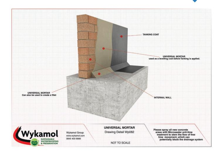
at the wall/floor joints and joints at the wall/wall.
