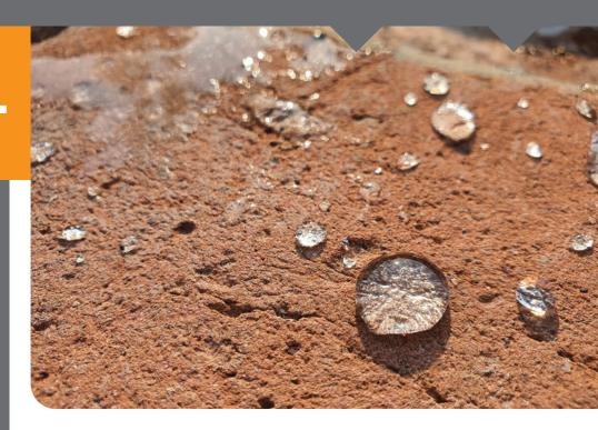
**DrySeal** is a, unique, thixotropic, water repelling masonry protection cream which can be used on a range of building materials. Dependent on the porosity of the substrate, the effective siloxane ingredient penetrates the substrate within a short period of time (30 minutes to several hours), where it reacts to become a permanent, chemically bonded, silicone coating.
