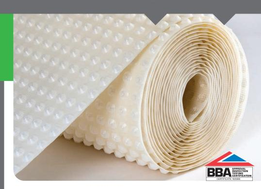
**CM8 Cavity Drain Mesh Membrane** is a 8 mm studded membrane incorporating a tough HDPE mesh lathing welded to the front face, allowing the direct application of various plaster finishes, adhesive 'dabs' and plasterboards and delivering a grade 3 environment to BS8102:2022 and NHBC Chapter 5.4.
