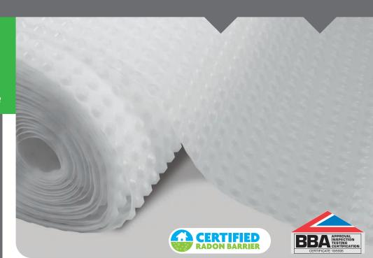
**CM8 HD** is an 8mm studded high density membrane suitable for type C waterproofing and delivering a grade 3 environment to BS8102:2022 and NHBC chapter 5.4. We recommend using the HD version on our Wykamol High Load insulated spacer and also in commercial areas where a more impact resistant membrane may be needed. CM8 HD is also an excellent radon barrier and has passed all the relevant tests for resistance to this gas.
