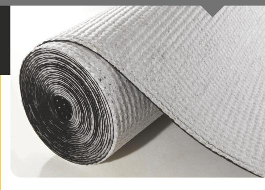
The dual layers comprise of the Wykamol 8mm studded HDPE membrane and a nonwoven geotextile manufactured from UV stabilised, high tenacity, virgin polypropylene fibres that have been mechanically entangled to provide high strength, high extensibility, high loft and excellent abrasion characteristics. The geotextiles are also thermally treated to reduce thickness while maintaining excellent mechanical properties.
