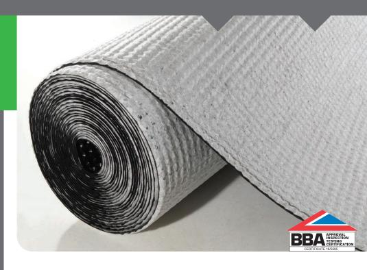
The dual layers comprise of the Wykamol 8mm studded HDPE membrane and a nonwoven geotextile manufactured from UV stabilised, high tenacity, virgin polypropylene fibres that have been mechanically entangled to provide high strength, high extensibility, high loft and excellent abrasion characteristics. The geotextiles are also thermally treated to reduce thickness while maintaining excellent mechanical properties.
